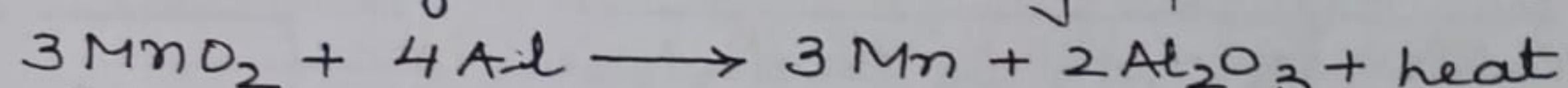
These reactions are highly exothermic. The amount of heat produced is so large that metals are obtained in molten state. e.g. the reaction of iron oxide with aluminium is used to join railway tracks or cracked machine parts. This reaction is known as THERMIT REACTION.
