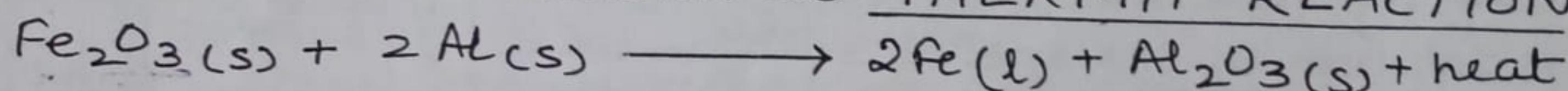
The molten iron is then poured between the broken iron pieces to weld them (or to join them). This process is known as ALUMINOTHERMY OR THERMITE WELDING.
